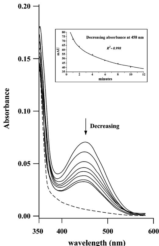
FIGURE 2: Photoactivation of 7,8-DMBC. The ring-opened product absorbs at a maximum wavelength of 458 nm and has a half-life of 14.8 min (inset). The spectrum of the sample before irradiation is also shown (---).
