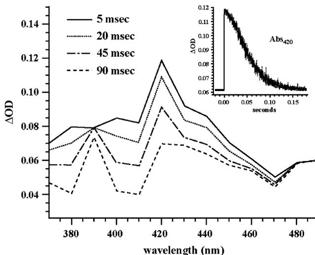
FIGURE 3: Detection of a ring-opened product upon irradiation of 5,6-DMBC in phosphate buffer by laser flash photolysis. The product reverts to starting material within 150 ms following multiphasic kinetics (inset).
