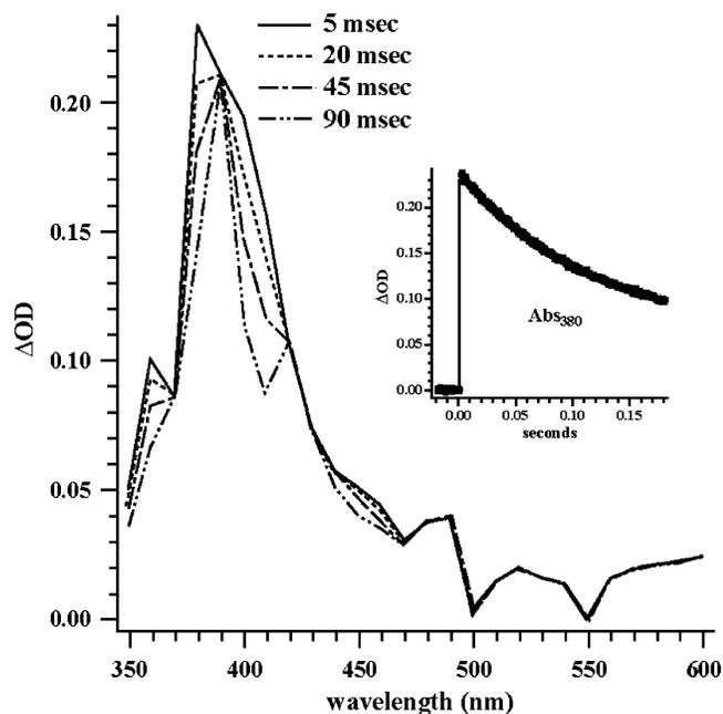
FIGURE 4: Photoactivation of precocene I in ethanol. The ring-opened product absorbs strongly at 380 nm and substantial amounts remain after 150 ms (inset).
