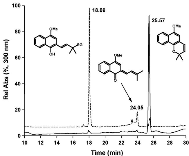
FIGURE 5: Reactivity of lapachenole with glutathione upon irradiation: (—) reaction mixture prior to photolysis; (---) reaction mixture after 5 min of irradiation. Almost all of the starting material is consumed and a single glutathione conjugate is detected.
