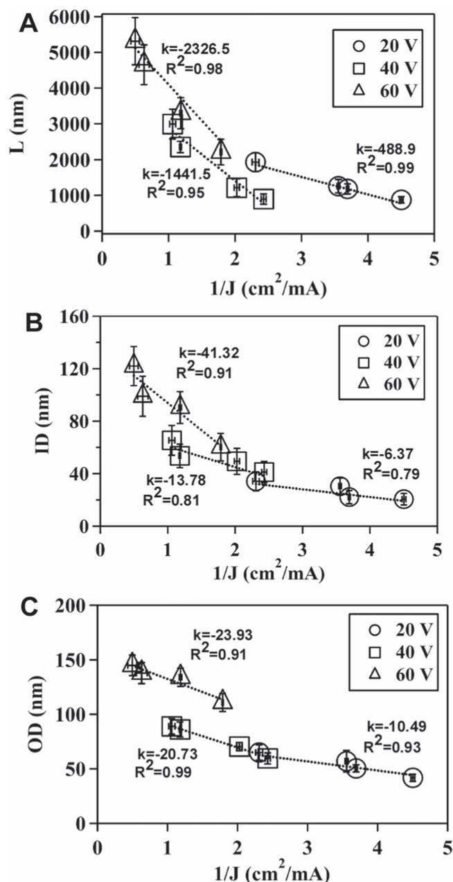
**Figure 4.** Inverse of the current density ( $J$ ) correlates linearly with the dimension of  $\text{TiO}_2$  nanotubes. The dependence of (A) length ( $L$ ), (B) inner diameter ( $ID$ ) and (C) outer diameter ( $OD$ ) of  $\text{TiO}_2$  nanotubes on  $1/J$  at an anodizing voltage of 20, 40, or 60 V.  $R^2$  is the correlation of determination and  $k$  is the slope of the linear regression fitting curve.
