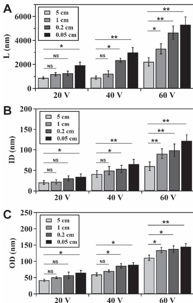
**Figure 2.** Effect of electrode distance ( $d$ ) on the growth of TiO<sub>2</sub> nanotubes at different anodizing voltages. The dependence of (A) length ( $L$ ), (B) inner diameter ( $ID$ ) and (C) outer diameter ( $OD$ ) of TiO<sub>2</sub> nanotubes on  $d$  at an anodizing voltage of 20, 40 or 60 V. \*\* $P < 0.01$ , \* $P < 0.05$ , and non-significant (NS) were calculated based on paired student's  $t$ -test analysis.
