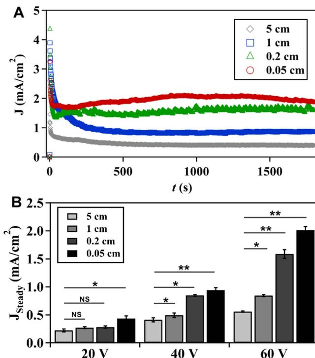
**Figure 3.** Electrode distance ( $d$ ) regulates current density ( $J$ ) during the anodic growth of TiO<sub>2</sub> nanotubes. (A) The typical change of current density with electrode distance when anodizing voltage is 60 V. (B) The dependence of steady-state current density on  $d$  at different anodizing voltages. \*\* $P < 0.01$ , \* $P < 0.05$ , and non-significant (NS) were calculated based on paired student's  $t$ -test analysis.
