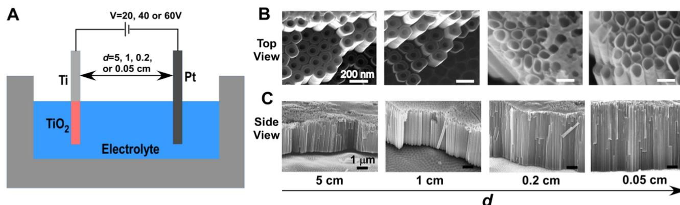
**Figure 1.** Electrode distance regulates the anodic growth of a TiO<sub>2</sub> nanotube. (A) Schematics of the anodic growth of TiO<sub>2</sub> nanotubes. The anodizing voltage ( $V$ ) is kept at 20, 40 or 60 V. The distance between the cathode (Pt) and anode (Ti) ( $d$ ) varies at 5, 1, 0.2, or 0.05 cm for each anodizing voltage. SEM images of (B) top view and (C) side view of TiO<sub>2</sub> nanotubes fabricated at 60 V when the electrode distance is controlled at 5, 1, 0.2, or 0.05 cm.
